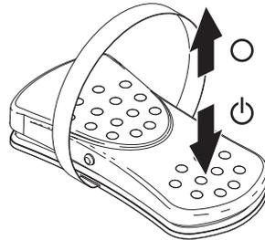
In wireless operation the flexible foot switch is supplied with voltage from a battery. If the battery power starts to fail, the orange PEDAL LED on the unit lights up.
