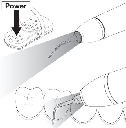
6 LEDs are integrated into the front section of the handpiece. The light conductor is located under the front cover. As soon as the flexible foot switch is operated and "Power" is selected on the operating panel, the LEDs light up. The LEDs go out approx. 4 seconds after the flexible foot switch is released.
